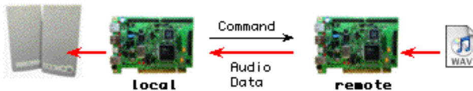
Figure 4-21: Playing a File from Another OTG Device on the Current OTG device
